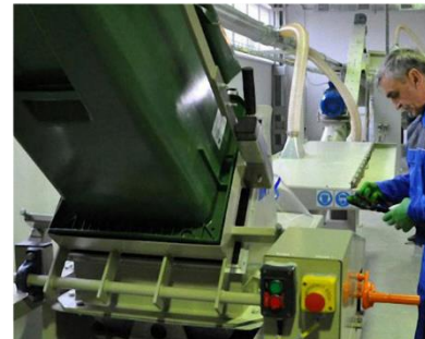
Figure 9.4. The decontamination equipment for mercury lamps and other items containing mercury vapor
