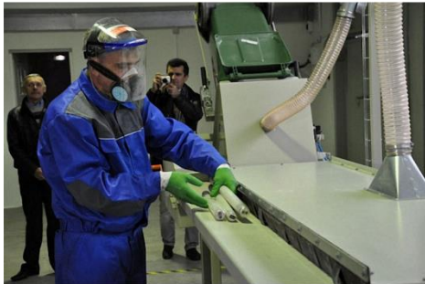
Figure 9.4. The decontamination equipment for mercury lamps and other items containing mercury vapor
